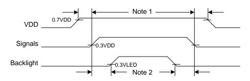
Fig. 8.7 Power Sequence Timing
