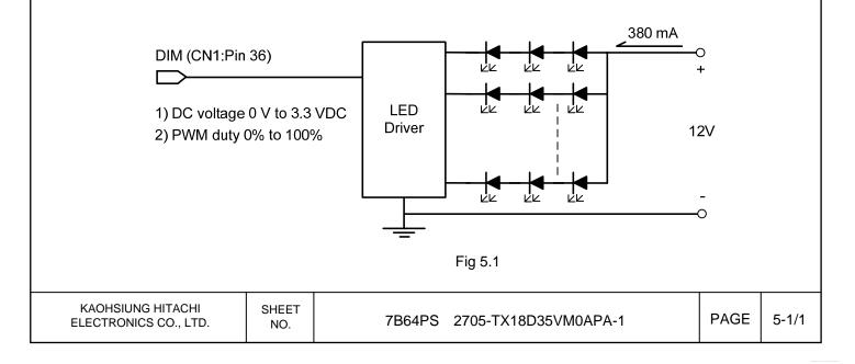
Note 2: Dimming function can be obtained by applying DC voltage or PWM signal from the display interface CN1. The recommended PWM signal is 1K ~ 10K Hz with 3.3V amplitude.
