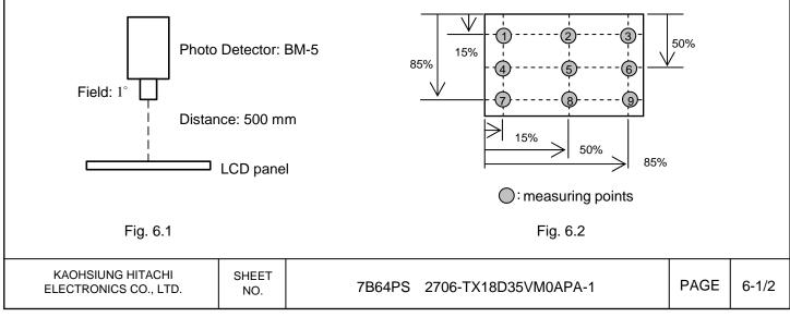
Note 3: The Contrast Ratio is measured from the center point of the panel, P5, and defined as the following equation:
