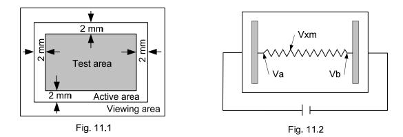
As shown in Fig. 11.2, applying voltage meter to measure Va, Vb and Vxm, where Va is the maximum voltage in the active area; Vb is the minimum voltage in the active area; Vxm is the measured voltage of point x selected by random. Afterwards, the linearity can be calculated by following equation:
